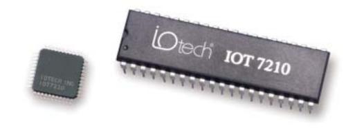
The IOT7210 is an enhanced replacement for the NEC µPD7210 IEEE 488 controller device
